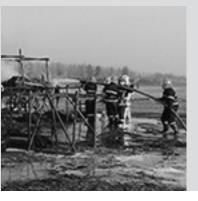
After a 4-minute preburn, the 3% F-500 Encapsulator Agent (F-500 EA) solution was applied utilizing two 500 l/min nozzles. The fire was extinguished after just 7 minutes.
